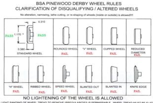
LIGHT SANDING OF WHEEL TREAD TO REMOVE IRREGULARITIES IS PERMISSABLE, WHEEL TREAD MUST BE FLATI MINIMUM WHEEL DIAMETER ALLOWABLE IS 1.170 INCHES. MINIMUM WHEEL VEIGHT OF EACH WHEEL IS 2.45 GRAMS.
